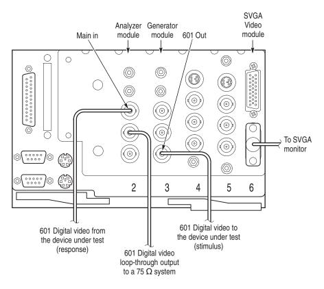
Figure 3–1: PQA 200 signal connections for serial digital signal testing
