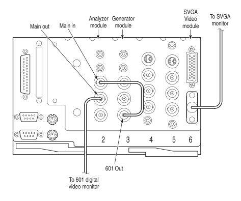
Figure C–1: Initial connections for the functional check
