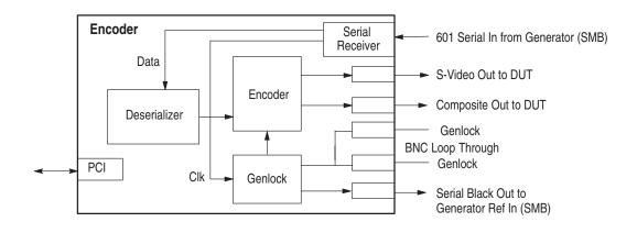
Figure 1–7: Encoder module connections
