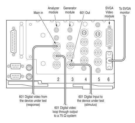
Figure 1–8: PQA200 signal connections for standalone serial digital signal testing
