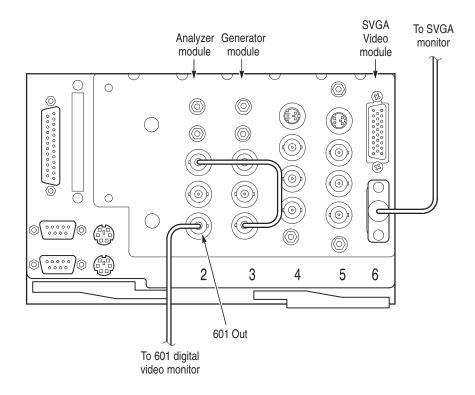
Figure C–2: Connection for analyzer 601 Out check
