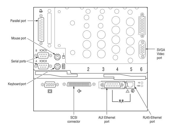
Figure 1–2: The rear panel of the PQA200 server
