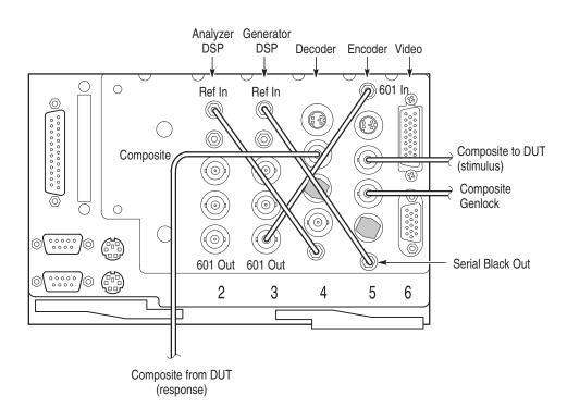
Figure 1–9: Option 01 connections using analog black burst genlock (lockup)
