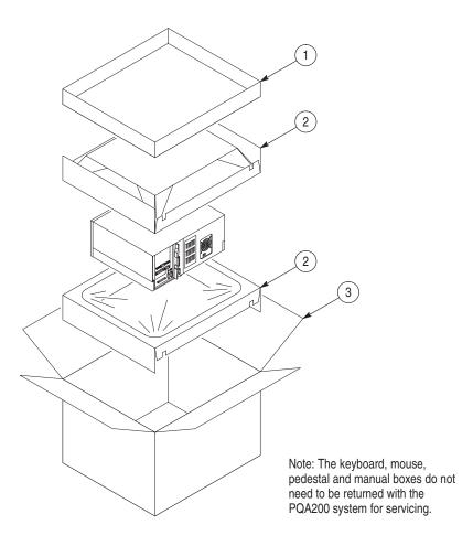
Figure D-1: Repackaging the PQA200 system server
