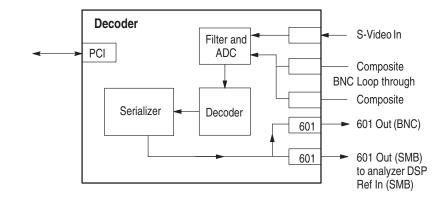
Figure 1–5: Decoder module connections
