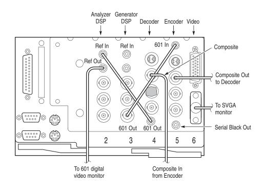
Figure C-4: Connections for the encoder and decoder functional check
