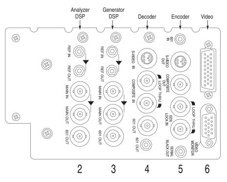
Figure 1–3: The PQA200 signal I/O ports with Option 01
