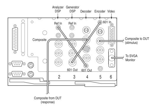
Figure 1–10: Option 01 connections using serial digital genlock (lockup)
